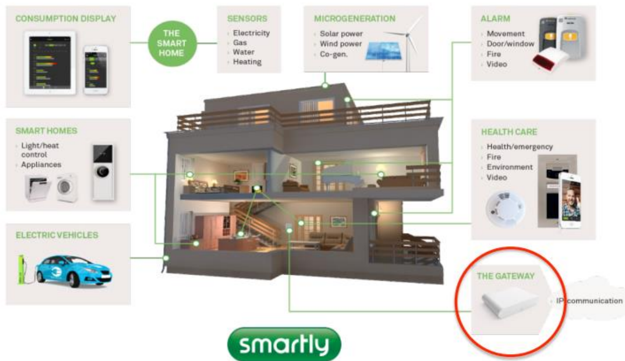
Figure ES-2. Functionality potentially enabled through Lyse Energi's home energy control system.
