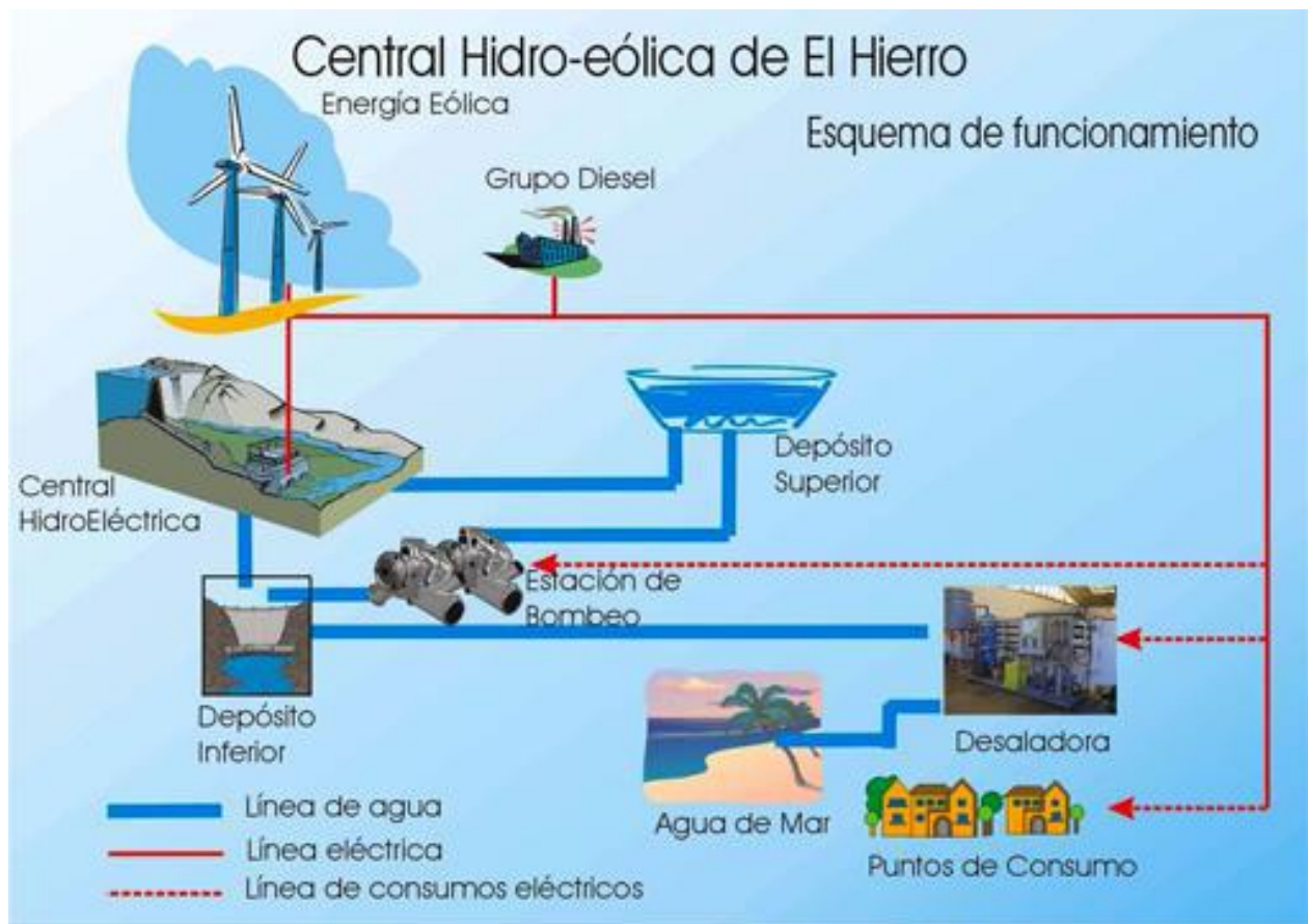
Figure 14. Hydro–wind plant schematics.
