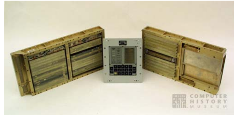
Apollo Guidance Computer (c. 1968) ~20k components; 8kB RAM; 16-bit ALU
