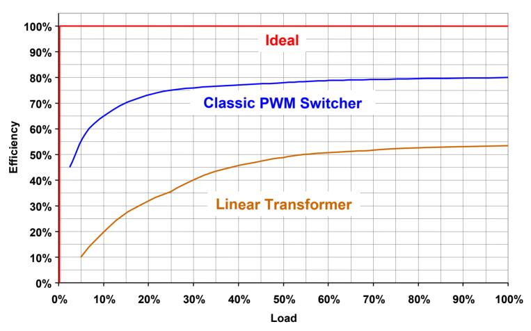
Switchers offer much higher efficiency at cost-parity with linears
