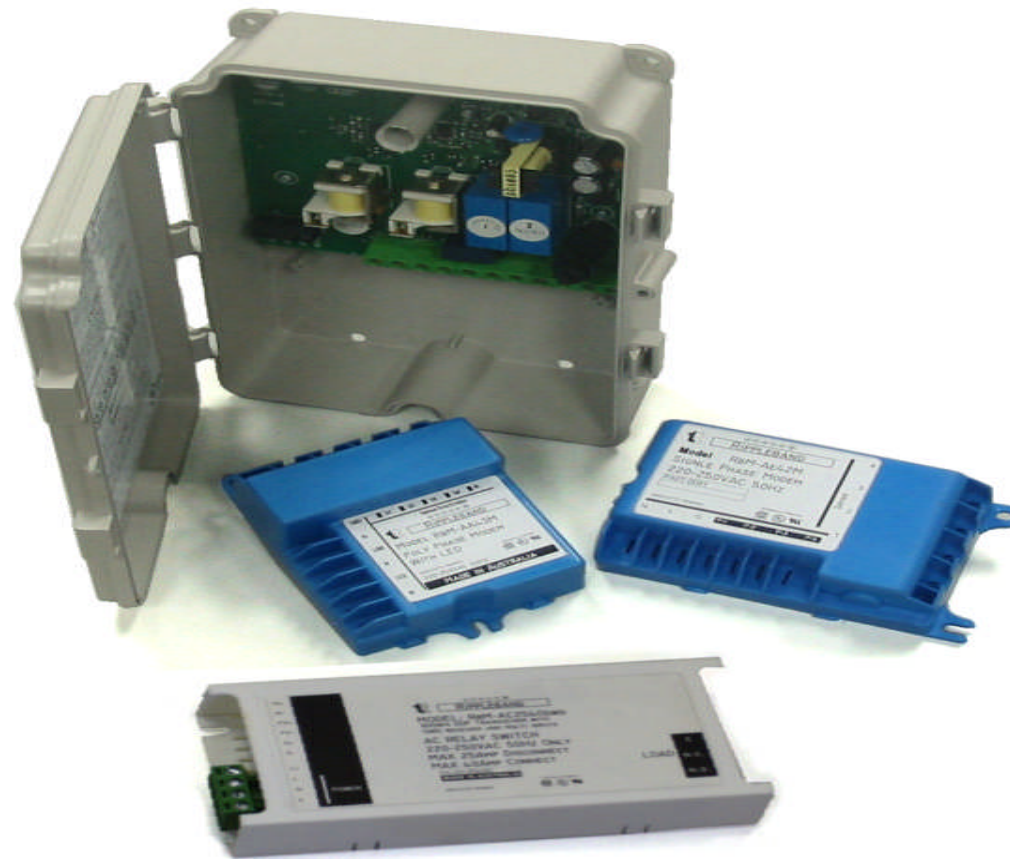
Phase 6/Tytronic Rippleband Neighbourhood Node, Load Agent and Meter Interfaces
