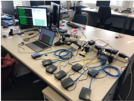
Testbench (11 RaspberryPi & Networking)
