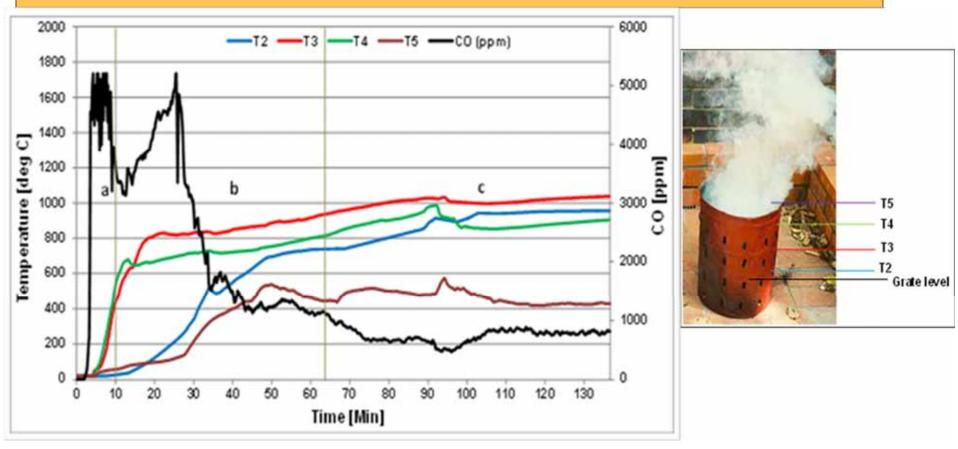
For the BLUD, ignition at the bottom creates an upward migrating pyrolytic zone that is starved of oxygen; generating a pyrolytic gas (CO, H<sub>2</sub>O, volatile and semi-volatile organic compounds), char and low flame temperatures (indicated by curve T5, Fig. 3, from 0 to 30 min after ignition).
