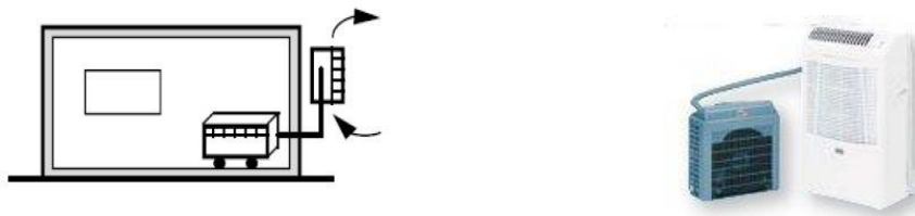
Figure 7. Non-ducted split-packaged units with mobile indoor unit
