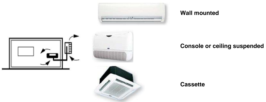
Figure 6. Non-ducted fixed split-packaged units
