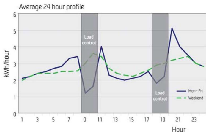
Fig. 8. Load profile for a household customer with hot water space heating system and RLC [13].
