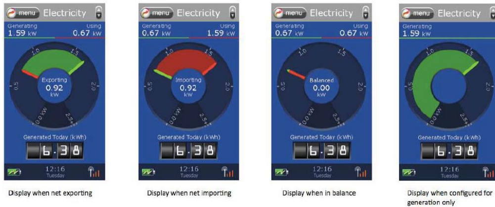
Figure 24: In-Home Display for Manual PV Balancing – Screen Display
