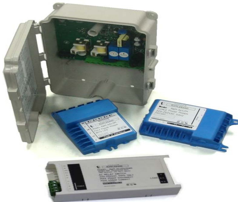
Figure A.20 Rippleband Neighbourhood Node, Load Agent and Meter Interfaces
