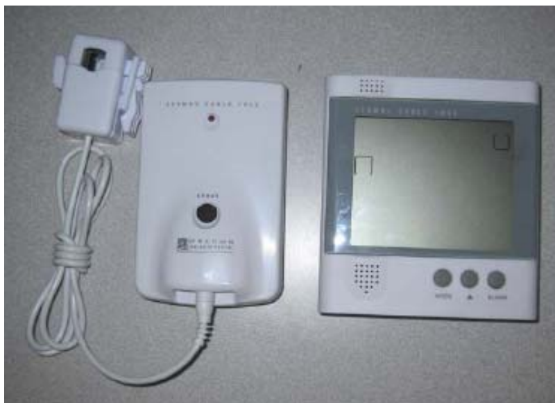
Figure A.2 Components of the Cent-A-Meter™
