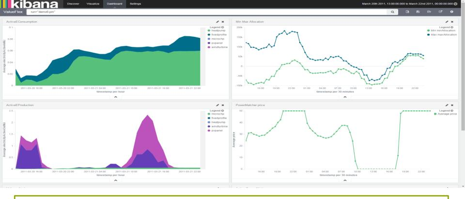
In this dashboard you see the consumption and production of all devices, the flexibility of the cluster as well as the 'PowerMatcher price' used by the PowerMatcher algorithm.
