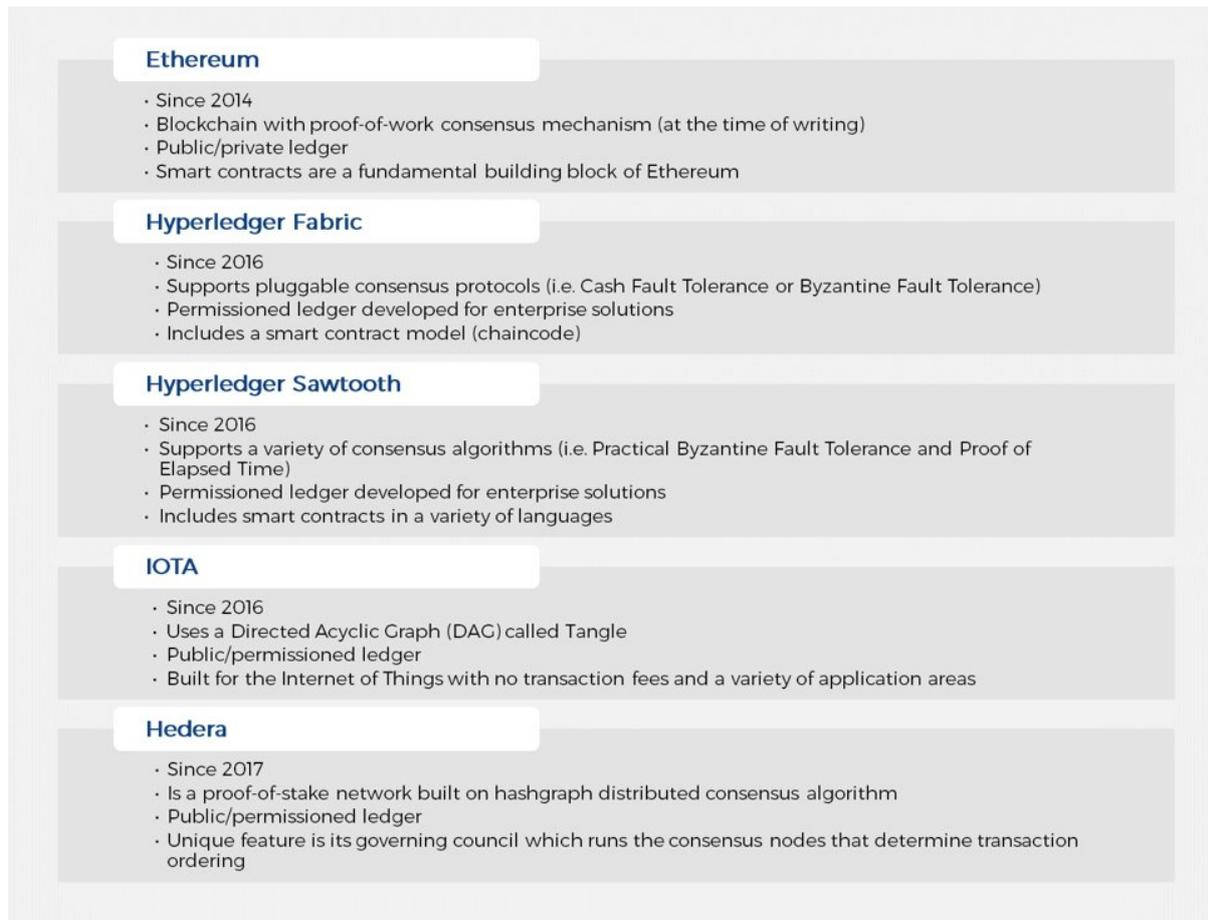
Figure 5 DLTs used in P2P energy trading pilot projects
