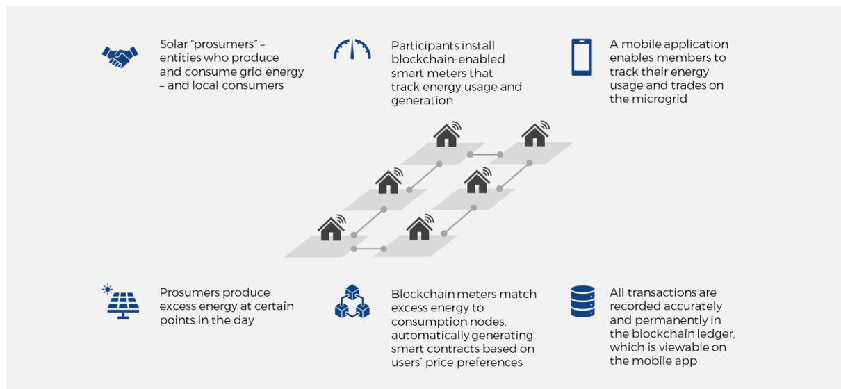
Figure 2 P2P energy trading using smart contracts (adapted from Henderson et al. (2018))
